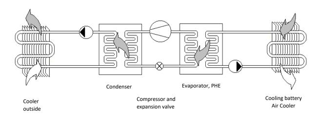
Temper's specific heat is lower than MPG or 1.3-Propanediol. However, its higher density leads to very similar values of volumetric flow. Together with the good thermal properties of Temper it results in smaller size and lower price of most of the system components, especially those that represent the highest cost in an installation, and consequently lower energy consumption.
